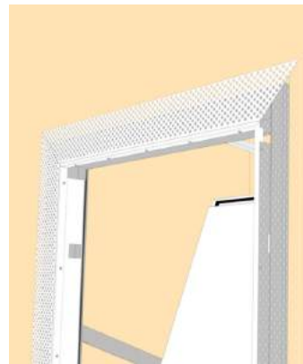
Skimmed finish and damper panel can then both be painted to match.
