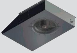
Colt Cyclone is a low profile, high velocity induction jet fan intended to control air movement and direct polluted air and smoke towards the extract positions in a car park or underground service area.
