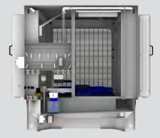
CoolStream S ventilates or cools as needed. In ventilation mode the system provides fresh outdoor air. On warmer days when pure ventilation is no longer sufficient the unit switches to evaporative cooling. The air temperature is then reduced via the process of evaporative cooling.
